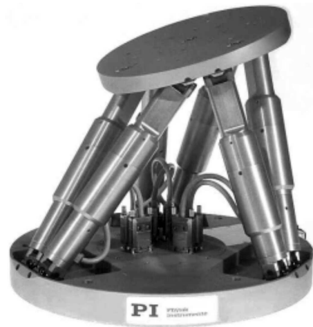
Figure 2.5: Example of a parallel six DOF manipulator (Physik Instrumente [19]).
